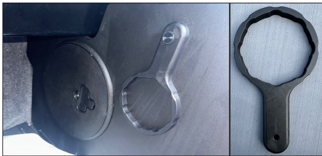
Sea Strainer Access Plate and Removal Tool.
