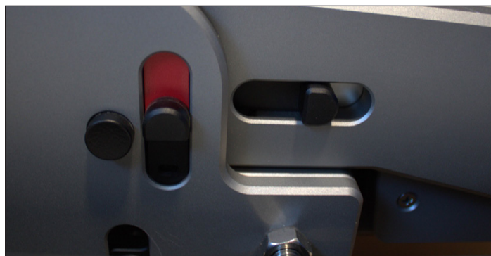
Max Pivot Seat Controls (on either side of cushion). From left to right: lock button, unlock tab, lean-back tab.
