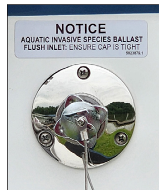
Ballast tank flush kit connection, located on starboard side of the transom.
