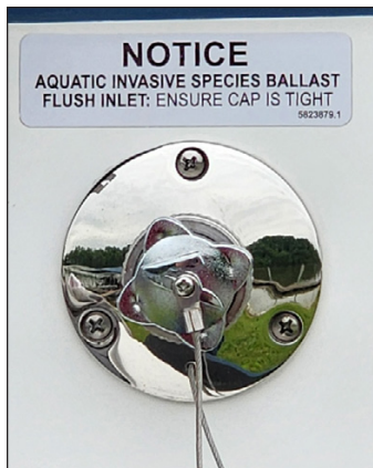
Ballast tank flush kit connector, located on starboard side of the transom.
