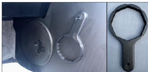
Sea Strainer Access Plate and Removal Tool.
