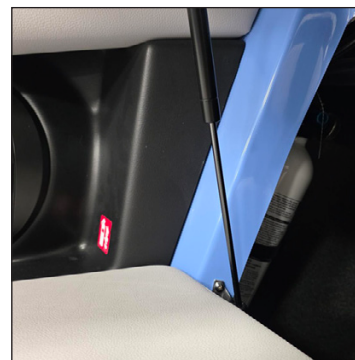
Mounted portable fire extinguisher. Note the nearby label.
