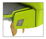
Surf Gate, especially when teamed with the Power Wedge III, offers the most innovative wake production in the industry. As with the Power Wedge III, control of the two transom-mounted gates is through dash buttons as explained in the *Dash and Displays* chapter of this manual. The Surf Gates can also be controlled by the optional Surf Band.
