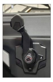
Note: The engine will not start unless the shifter/throttle control is in the Neutral position!
