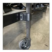
The trailer is equipped with a trailer jack designed to hold and lift the trailer into position when lowering onto the hitch ball of the tow vehicle. The jack is also useful for assisting and balancing whenever the trailer is free of the tow vehicle.
