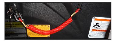
Your boat is equipped with an Emergency Safety Lanyard (cutoff switch). It is required by law that the lanyard be secured to the operator, and the lock plate attached to the Emergency Safety Lanyard, prior to starting the engine and anytime the engine is operating.
