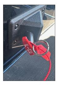
The boat is equipped with a fixed manual/automatic fire extinguisher system located in the engine compartment. In the event the system's sensor recognizes extreme heat in the compartment, the system will emit a chemically fixed suppression material.
