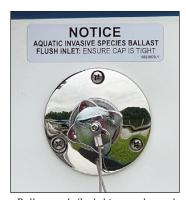
Ballast tank flush kit port, located on starboard side of the transom.
