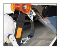
The bow safety strap is a secondary point of security in case the bow winch should fail or not be secured properly. Where installed and used, be sure to attach the clip to the bow eye of the boat.
