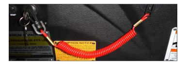
The Emergency Safety Lanyard attaches to the boat operator by way of a lanyard for the purpose of shutting off the engine if the operator, for any reason, moves or is moved away from the driver's helm.
