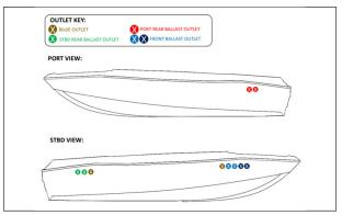
Figure 2: Axis Outlet Diagram
