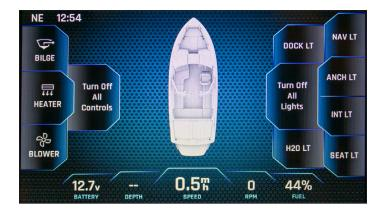
The *Lighting and Controls* screen allows the operator to control the boat's lights and other onboard devices. There is also a boat image that graphically shows where these lights or devices are at when turned ON.
