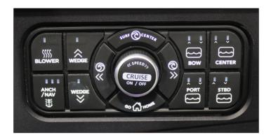
The boat may be equipped with the Sport Dash keypad (located to the right of the steering wheel, below the 7" display), which allows the operator convenient controls for the blower, navigation/anchor lights, Surf Gates, cruise control, Power Wedge, and ballast system.
