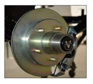
The system has several unique features not found on conventional trailer axles. Every possible leak point on the front and rear of the hub is sealed. (The slight pressure inside the hub is needed to keep water out of the hub chamber when the hub is submerged underwater during loading and unloading).
