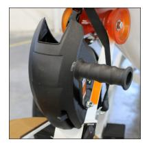
The trailer winch is a manually operated device to assist loading the boat onto the trailer and maintaining it in position for proper towing. The following information is important in assuring control and protection for you and the boat:
