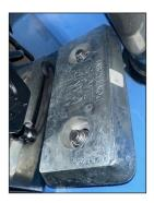
The purpose of an anode is to be sacrificial. There is a greater degree of attraction between the anode's metal and the corrosive action of the saltwater than between the boat's metal parts and the water. In the most simplistic terms, both rust (oxidation) and metal reduction are the effects of operating in saltwater. To reduce these naturally occurring results on boat components, the sacrificial anodes attract and reduce most of the effects.
