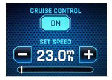
The engine must be running and in Neutral for the *Cruise Control* system to engage.
