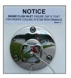
The engine flush kit is used to clean out the raw water pickup and operational areas of the engine. The kit attachment is located on the port side of the transom.
