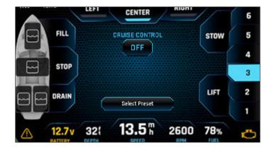
The Watersports Screen will show the driver the information about the Ballast System, Surf Gates, Wedge, Cruise Control, and Rider Profiles.
