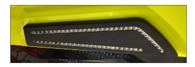
These are an option that offer additional visual assistance. The lights are located around the bow area and provide white light to the front of the boat. The docking lights are operated from a screen icon. On all models, the control is ON-OFF.
