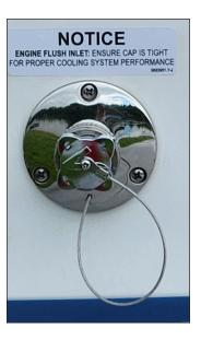
The flush kit is used to clean out the raw water pickup and operational areas of the engine. The engine flush kit attachment is located on the port side of the transom.
