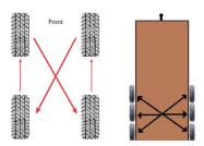
Rotating tires from front to back and from side to side can reduce irregular wear (for vehicles that have tires that are all the same size). The generally recommended rotation period is every 5,000 miles.
