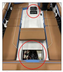
Fill pump valves and bilge T-handles are accessible through the fore and aft access panels (shown above, circled in red).
