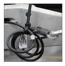
In addition to safety cables, the trailer is also equipped with a surge brake breakaway cable. The breakaway cable should be attached as tautly as possible but still allow for turning, including close quarters turns. The breakaway cable should **NEVER** be used as a substitute for braking or as a parking brake.
