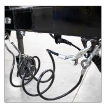
The trailer's safety cables can prevent the trailer from totally disengaging from the hitch. If it becomes necessary to replace the cables, ensure that the replacement cables:
