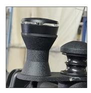
All boats equipped with towers will also have a 360-degree light on top for use at anchor. If the boat is operated in darkness, use the anchor light in accordance with local law and ordinances. This light is on whenever the navigation/anchor lights are on.
